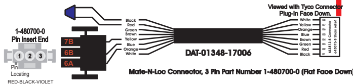
Mate-N-Loc Connector, 3 Pin Part Number 1-480700-0 (Flat Face Down) Mate-N-Loc Connector Operates Aux. 1, Aux. 2 & Heat on RCT-01490 or RCT-01507 from J3 on RCT-01492 or RCT-01493. Black & Red Operates Aux.3 with "Ignition".
